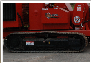
TRACK UNDERCARRIAGE Caterpillar 312B track drive system
