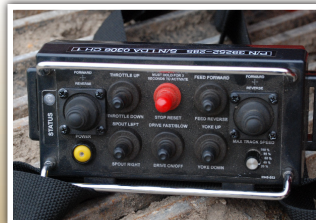
REMOTE CONTROL 15-function radio remote control with tethered back-up system
